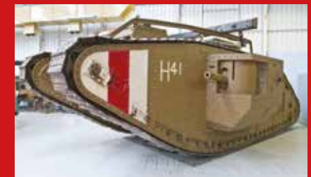
British Mark V tank. The Mark V entered service in 1918 and was a far more reliable and improved version of the Mark I of 1916 and Mark IV of 1917. It was armed with four machine guns and two 6 pounder guns. Bovington Tank Museum
