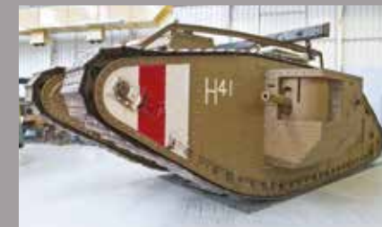
British Mark V tank. The Mark V entered service in 1918 and was a far more reliable and improved version of the Mark I of 1916 and Mark IV of 1917. It was armed with four machine guns and two 6 pounder guns. Bovington Tank Museum
