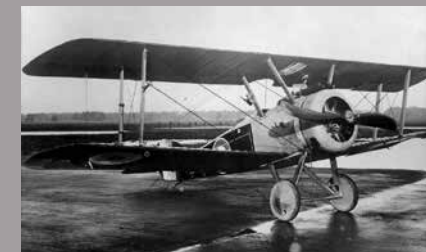
A Sopwith Camel of the Royal Flying Corps. The Camel was primarily a fighter designed to shoot down enemy aircraft, but it could strafe enemy trenches with its guns or carry light bombs under the wings.
